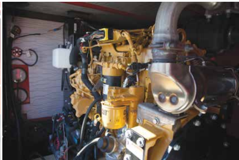
Since MagFan heaters don't use flames or liquids and have very few moving parts, maintenance is limited to the lubrication of three easily accessible grease points and oil changes every 500 to 1,000 hours.
