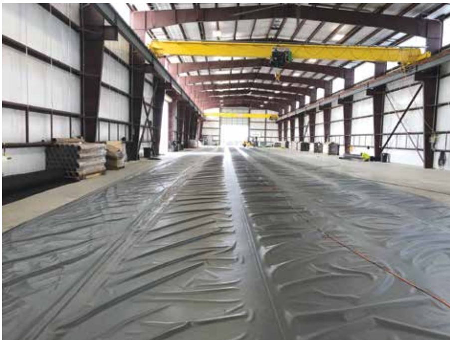
Custom fabricated geomembrane panels ready to be packaged and shipped for base layer soil contamination protection.
