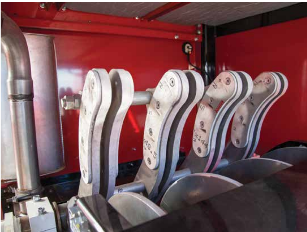
Precision Equipment Manufacturing's line of patented MagFan heaters use magnets and an axial-flow fan to generate a 200-degree temperature rise heat at up to 8,400 cubic feet per minute, without sparks, flames, friction, or liquids.
