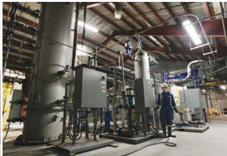
CE's pilot plant pellet reactor and associated equipment.
